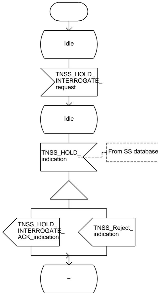
Figure 2: SS-HOLD, overall SDL for interrogation
